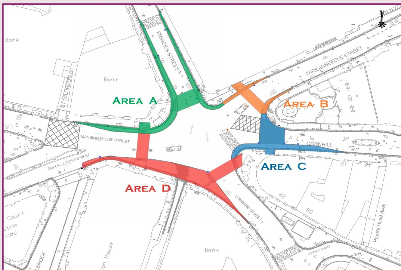
Image showing proposed widening of footways and crossings at Bank junction
